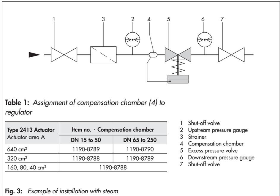
This mounting position must be adhered to; otherwise the safe functioning of the excess pressure valve cannot be guaranteed.
